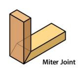
A mitre joint is a joint made by cutting each of two parts to be joined, across the main surface, usually at a 45° angle, to form a corner, usually to form a 90° angle, though it can comprise any angle greater than 0 degrees.
